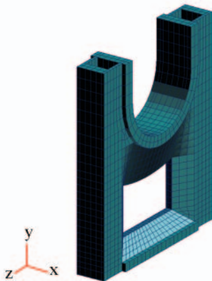
Fig. 2. Main bearing frame of Sulzer 7 RTA 84 C engine .
