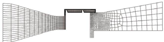
Fig. 5 Cross-section through geometrical model of 'isolated' seal
