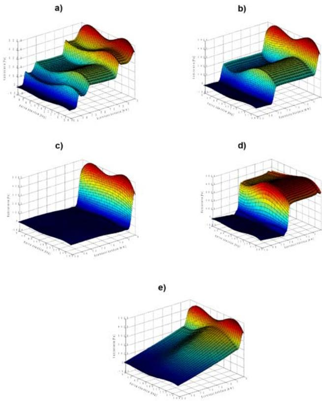
**Fig. 13** Pressure distribution in the seals: **a)** U4, **b)** U2, **c)** U1, **d)** U1s, **e)** U0 -for 20kPa working medium overpressure at inlet to turbine stage, and the rotor angular frequency equal to 566 rad/s
