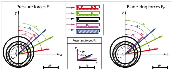
**Fig. 14** Vectors of: the pressure force  $F_C$  (on the left), blade-ring force  $F_W$  (in the middle) and resultant force  $F_P$  (on the right), acting on the rotor, for the model IV at 20kPa inlet overpressure and the rotor angular frequency of 566 rad/s (red colour stands for the seal U4, green – the seal U2, black– the seal U1, violet– the seal U1s, blue– the seal U0)
