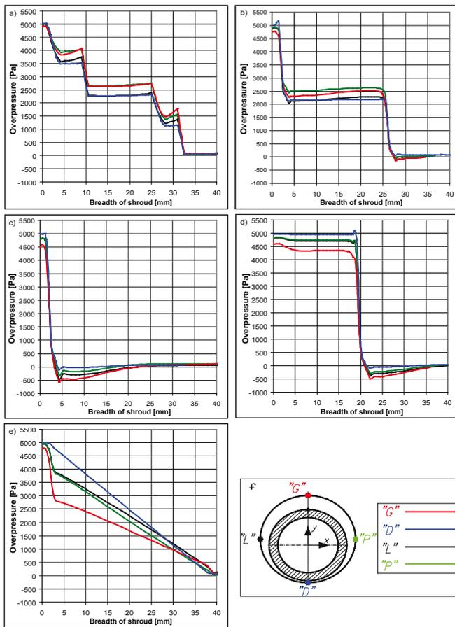
**Fig. 10** Pressure distribution in the seals along shroud breadth for viscous working medium and the shroud angular frequency equal to 566 rad/s: a) U4, b) U2, c) U1, d) U1s, e) U0 (f – arrangement of the cross-sections along seal circumference)
