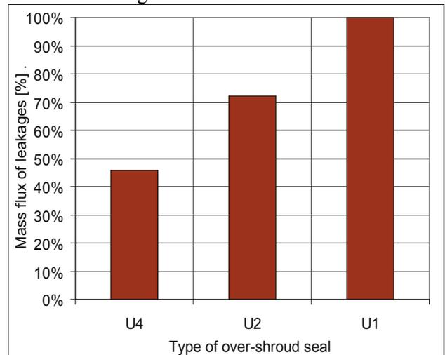
**Fig. 16** Mass flux of leakages flowing through the seal U4, U2 and U1 at the rotor angular frequency of 566 rad/s and 20kPa overpressure of working medium at inlet (the values are related to the mass of leakage from the single-tooth seal U1)
