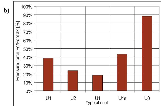
**Fig. 11** Vectors, (a), and values, (b), of the pressure force FC occurring in the investigated seals for viscous working medium and the shroud wall angular frequency equal to 566 rad/s (the force values are related to that which occurs in the U0 seal of motionless shroud)
