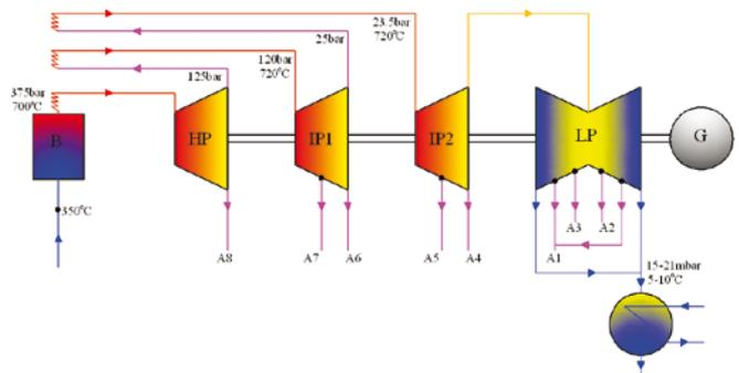
Fig. 3 Simplified schematic diagram of THERMIE 700 steam cycle
