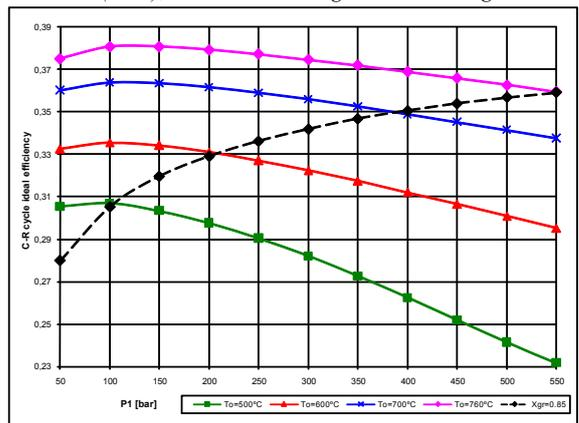
**Fig. 7** Relation of Clausius-Rankine cycle efficiency (with steam wetness degree taken into account according to Bauman formula) in function of fresh steam pressure and temperature at condenser internal pressure kept constant (4kPa), and the wetness degree limit curve  $x_{gr}=0.85$
