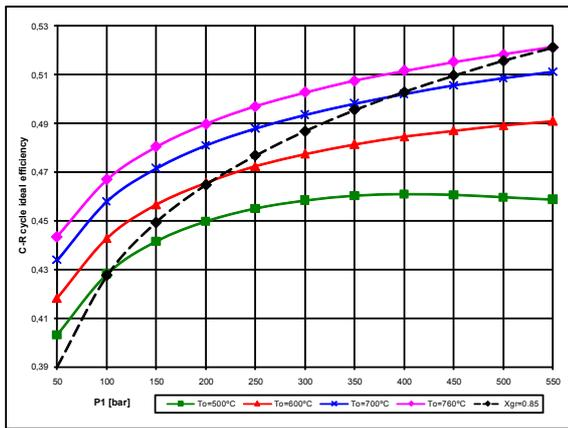
**Fig. 5** Relation of ideal efficiency of Clausius-Rankine cycle in function of fresh steam pressure and temperature at condenser internal pressure kept constant (4kPa), and the wetness degree limit curve  $x_{gr}=0.85$
