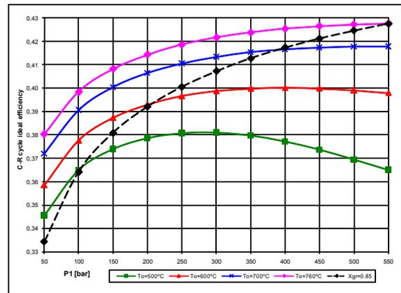
**Fig. 6** Relation of real efficiency of Clausius-Rankine cycle in function of fresh steam pressure and temperature at condenser internal pressure kept constant (4kPa), and the wetness degree limit curve  $x_{gr}=0.85$
