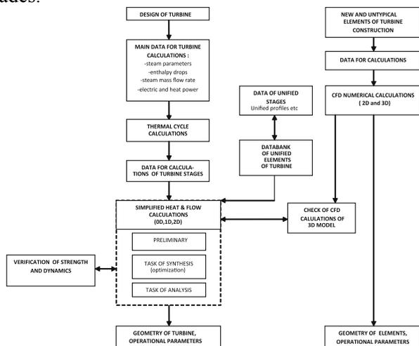
Fig.7 CAD system for high-loaded turbine stages, acc. [6].
