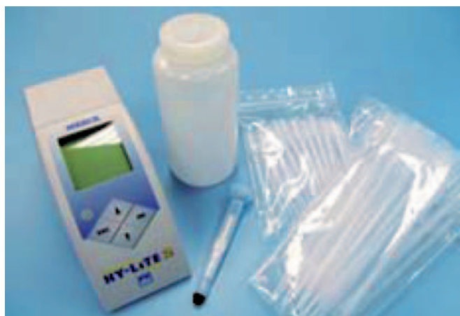
Fig. 3. Hy-Lite device (prod. Merck) used in ATP method for microbial contamination assessment.
