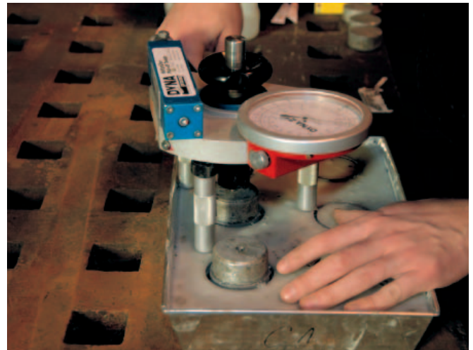
Fig. 8. Measurements of adhesion of concrete filler to protective barrier
