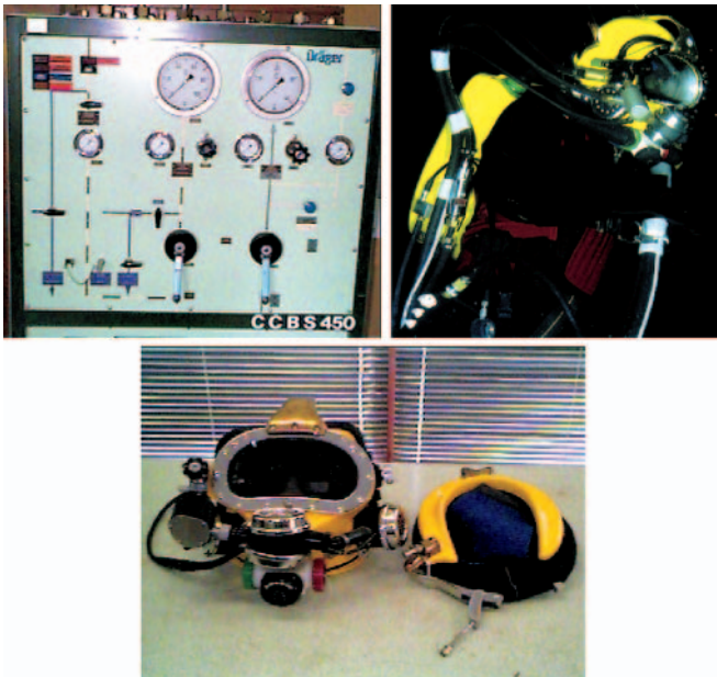
Photo 37. Main board and the diver's hose-mix-CCR system CCBS type
