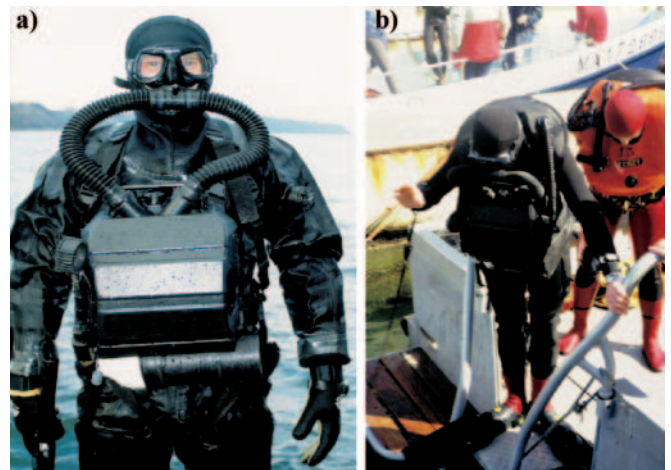
Photo 34. oxy-CCR Oxy-NG type. a) during sea tests (the own photo), b) the author during trials in the harbour basin of Marseill
