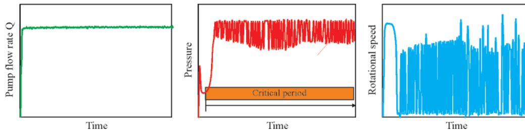
**Fig. 14.** Time-histories of parameters characteristic for incorrect motor operation (area C in Fig. 10).
