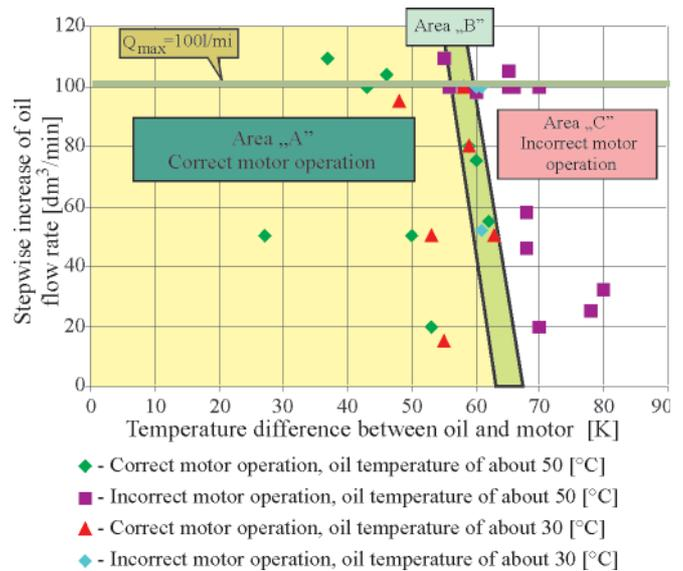
Fig. 18. Areas of operating parameters of SOK 100 satellite motor in thermal shock conditions
