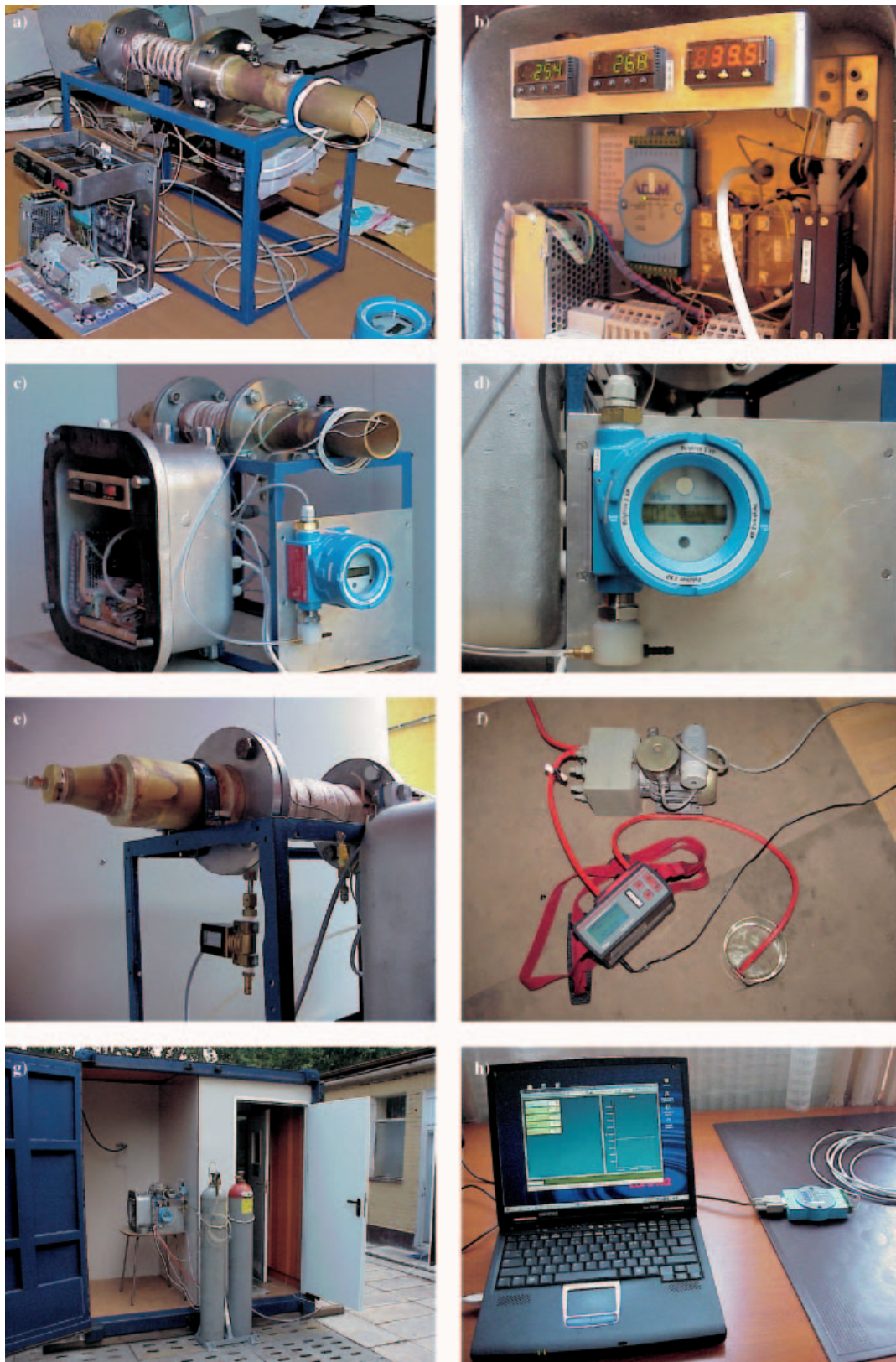
Fig. 2. The test stand and reactor's instrumentation: a) reactor and control panel; b) control panel; c) testing system; d) POLYTRON 2XP analyzer; e) inlet of gas for reaction; f) suction pump and MULTIWARN multi-channel analyzer; g) test stand; h) recording system for test results
