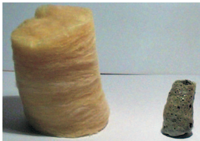
Fig. 9. The view of mineral wool sample before and after the fire tests
