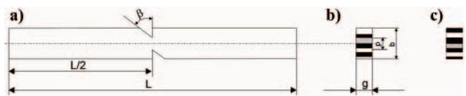
Fig.2. a) modified Iosipescu specimen, b) specimen with summer wood upper layers, c) specimen with spring wood upper layers. \beta = 45^\circ , g = 5 mm - specimen thickness, b = 20 mm - specimen width, p = 5 mm - length of measuring section, L = 80 mm - specimen length
