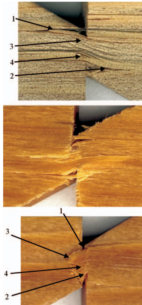
Fig. 6. Specimen crack patterns: a) natural wood, b) composite D-PMM K0.35, c) composite D-PMM K0.56 (1, 2, 3, 4 - successive stages of wooden specimen crack)
