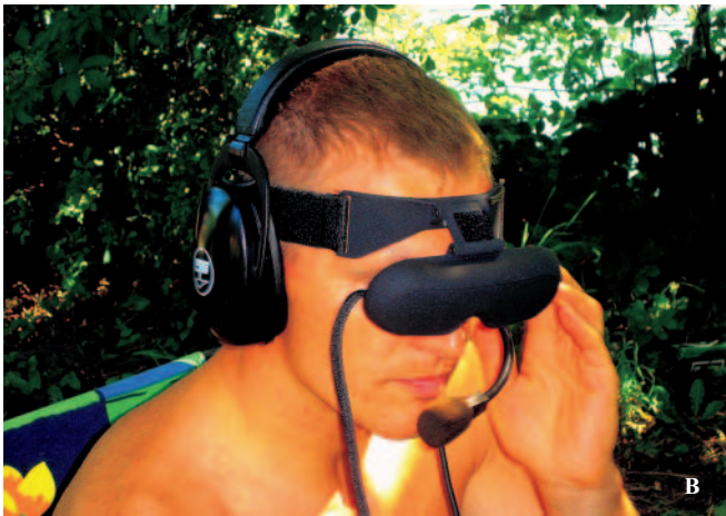
Fig. 11. System of three-dimensional visualisation of underwater objects: A – underwater part of the system during basin tests, two-camera system of picture acquisition in DVD quality, laser subsystem for placing background points to the frame to allow its scaling and dimensioning, B – element of surface part of the system – subsystem for head-located visualisation, operator is equipped with special goggles and receives a non-compressed picture from two cameras, to each eye separately [13].
