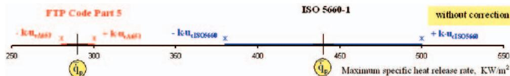
Fig. 2. Heat release rates obtained for wool carpet using ISO 5660-1 and FTP Code Part 5 (Res. A. 653 (16)) methods, and taking into account measurement uncertainties ( $k_u$  – extended uncertainty)
