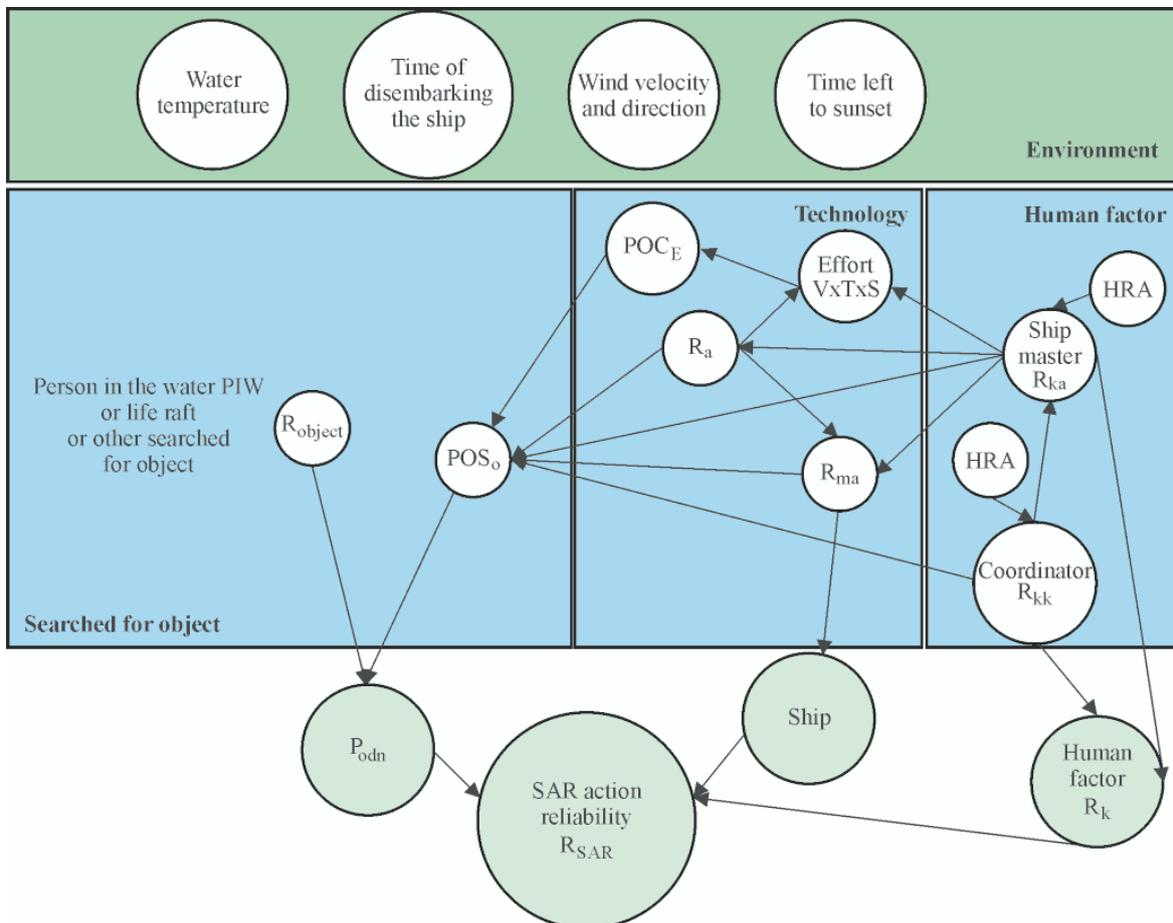
Fig. 2. The bayesian network for one search ship and one searched for object
