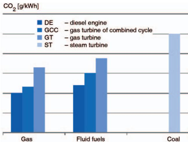
Fig. 1. Specific emission of CO<sub>2</sub> contained in exhaust gases for various types of electric power stations and mineral fuels [14]
