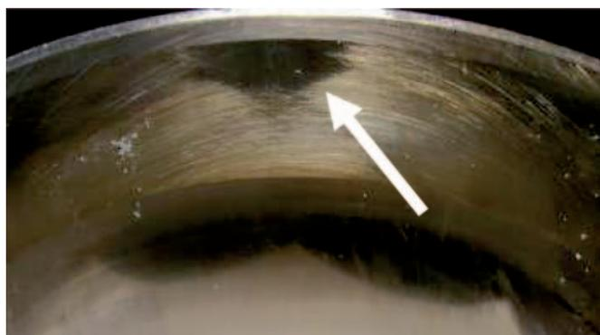
Fig. 7. Polished (mirror) cylinder bearing surface
