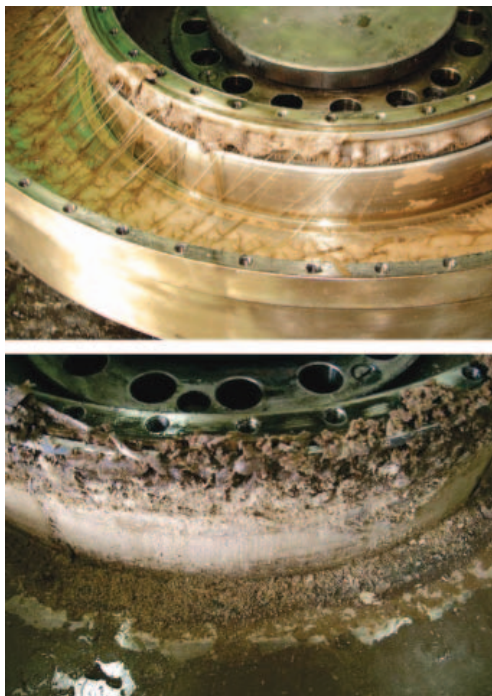
Fig. 8. Used silicone oil (solidified material) stuck to the casing of the viscous torsional vibration damper
