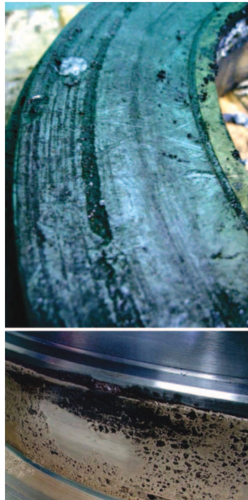
Fig. 10. Failures of inner surfaces of a viscous torsional vibration damper
