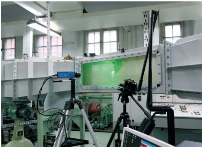
Fig. 2. Cavitation tunnel during PIV measurements
