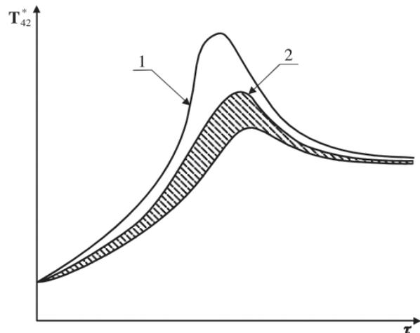
Fig. 5. Hypothetical time-histories of exhaust gas temperature changes during turbine engine start-up (acceleration) – the hatched area represents the range of correction of the measuring thermocouple inertia: 1 – real temperature, 2 – measured temperature
