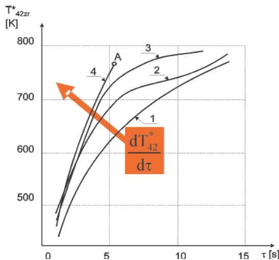
**Fig. 2.** Exhaust gas temperature changes recorded behind TNC of a three-shaft engine with a separate power turbine vs. start-up time: 1 – brand-new engine; 2 – engine in third year of operation; 3 – engine after five years of operation; 4 – unsuccessful engine start-up after five years of operation; A – automatic engine shut-down
