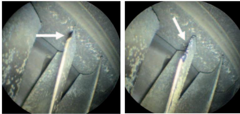
Fig. 6. Partly burned high-pressure turbine rotor blade tips
