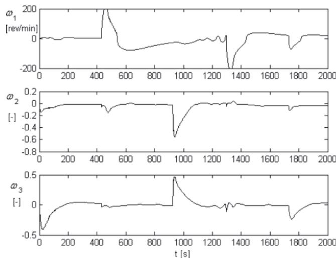
Fig. 11. Simulation results – computed propeller angular velocities by the allocation algorithm  $\omega_1$  - desired rotational velocity of the main propeller,  $\omega_2$  - desired rotational velocity of the tunnel thruster mounted at the bow,  $\omega_3$  - desired rotational velocity of the tunnel thruster mounted at the stern
