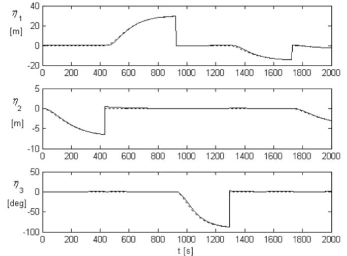
Fig. 7. Simulation results – the solid lines represent positions while the dashed lines represent reference (r-frame)  $\eta_1 = x$  - position  $x$ ,  $\eta_2 = y$  - position  $y$ ,  $\eta_3 = \psi$  - heading
