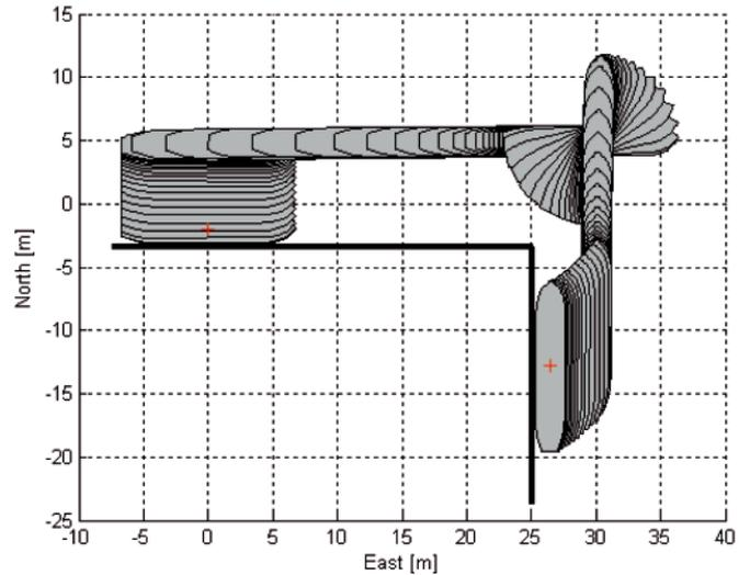
Fig. 6. Simulation results - example ship motion trajectory
