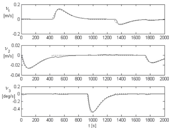
Fig. 8. Simulation results – the solid lines represent velocities while the dashed lines represent references (b-frame)  $v_1 = u$  - surge,  $v_2 = v$  - sway,  $v_3 = r$  - yaw rate
