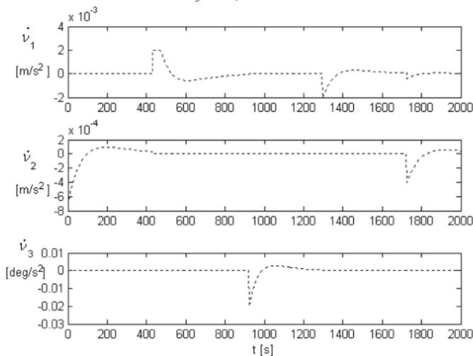
Fig. 9. Simulation results – the dotted lines represent set accelerations (b-frame)  $\dot{v}_1 = \dot{u}$  - surge,  $\dot{v}_2 = \dot{v}$  - sway,  $\dot{v}_3 = \dot{r}$  - yaw
