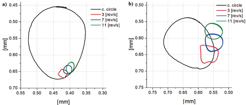
**Fig. 9.** Shaft orbits measured on both sides of the bearing with polymer bush, under load of 0.4 MPa; **a)** left side of the bush, **b)** right side of the bearing; orbits for three successive shaft revolutions
