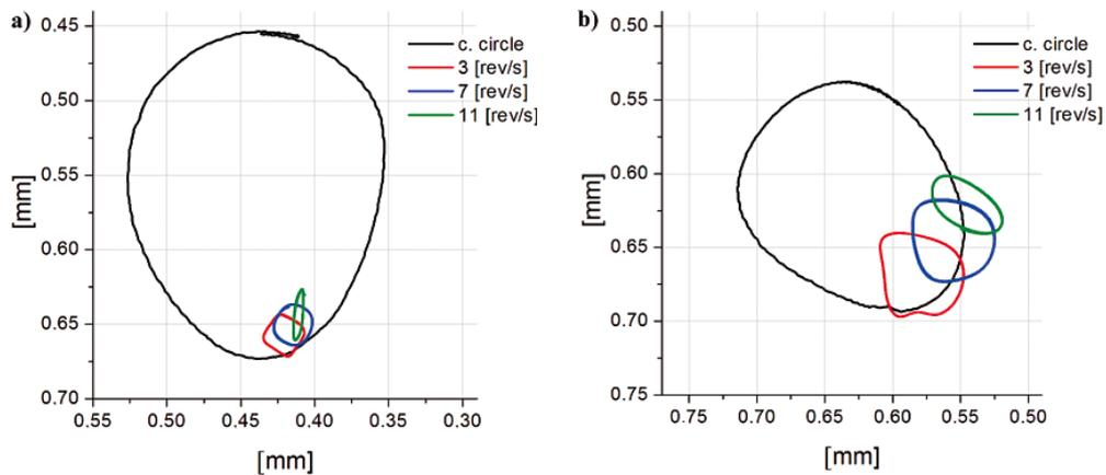
**Fig. 10.** Shaft orbits measured on both sides of the bearing with polymer bush, under load of 0.6 MPa; **a)** left side of the bush, **b)** right side of the bearing; orbits for three successive shaft revolutions
