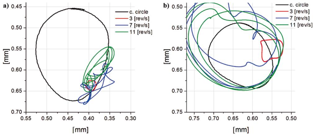
**Fig. 8.** Shaft orbits measured on both sides of the bearing with polymer bush, under load of 0.2 MPa; **a)** left side of the bush, **b)** right side of the bearing; orbits for three successive shaft revolutions
