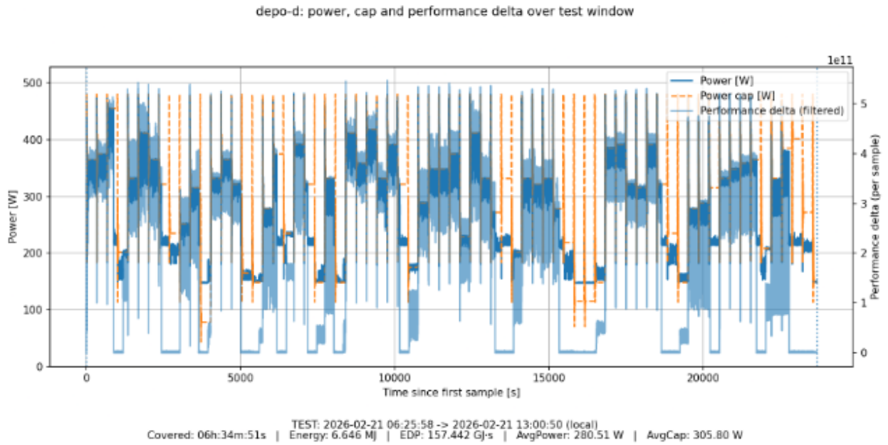
Figure 9: Power consumption profile during the first 12 hours of execution with depo-d optimizing the Energy metric on AMD EPYC 9334.
