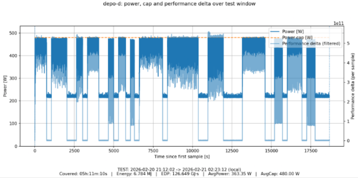
Figure 8: Power consumption profile during the first 12 hours of execution without power capping on AMD EPYC 9334.
