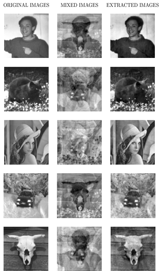
Figure 6. Computer simulation results for a mixture of image signals: original, mixed and extracted images (set of test images used in [16])
