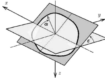
**Figure 4.** A surface section corresponding to the formula of surface parameterization (1)
