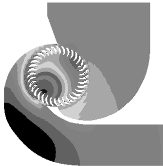
Figure 8. The static pressure contour plot including the eccentric vortex region
