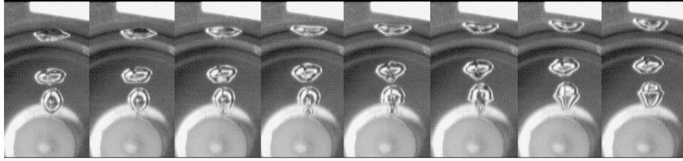
**Figure 8.** Incipient coalescence of bubbles during bubble formation from an orifice 0.3mm in diameter; average gas flow rate – 0.83mL/s; time resolution – 1000fps
