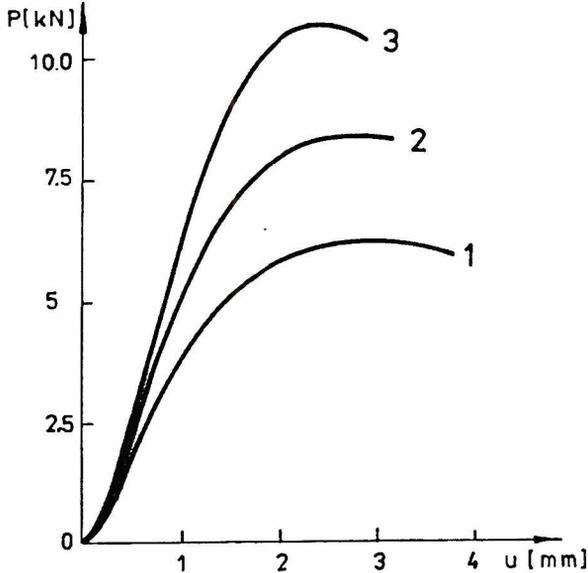
**Figure 7.** Numerical results for sand anchors in rock (axisymmetric case): pull-out force  $P$  against the vertical anchor displacement  $u$  ( $r_w = d_{50}$ ,  $e_0 = 0.6$ ,  $k = \infty$ ): 1)  $d_{50} = 0.5$  mm,  $d_r = 15.4$  mm, 2)  $d_{50} = 0.5$  mm,  $d_r = 23.8$  mm, 3)  $d_{50} = 1.0$  mm,  $d_r = 23.8$  mm
