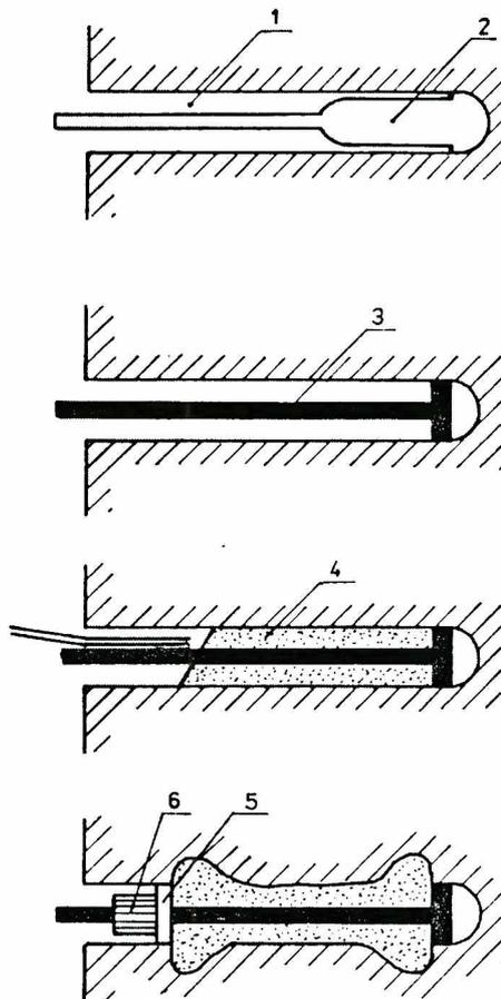
**Figure 4.** Installation of granular anchors in soils [14] (1. borehole, 2. drill, 3. rod with an end plate, 4. dense granulate, 5. head plate, 6. nut)
