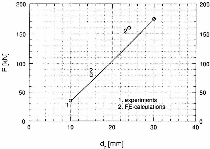
**Figure 9.** Calculated maximum pull-out force  $F$  against the diameter of the anchor rod  $d_r$  for fine gravel in rock ( $d_{50} = 2.8$  mm,  $d = 37.7$  mm)
