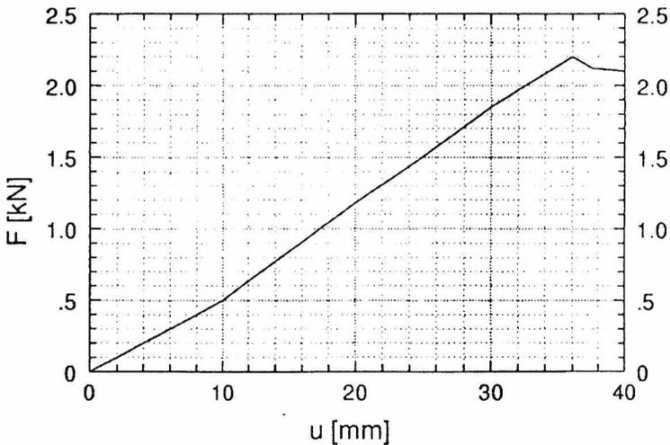
**Figure 10.** Calculated pull-out force  $F$  against the vertical displacement of the anchor rod  $u$  for gravel in silt ( $d_{50} = 4$  mm,  $l = 0.3$  m,  $d_r = 24$  mm,  $d = 80$  mm)
