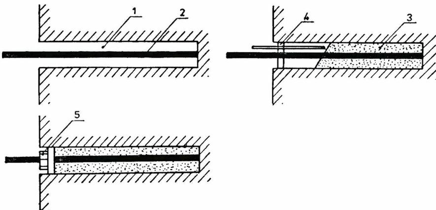
Figure 1. Construction of granular anchors in rock [14] (1. borehole, 2. steel rod, 3. dense sand, 4. head plate, 5. nut)
