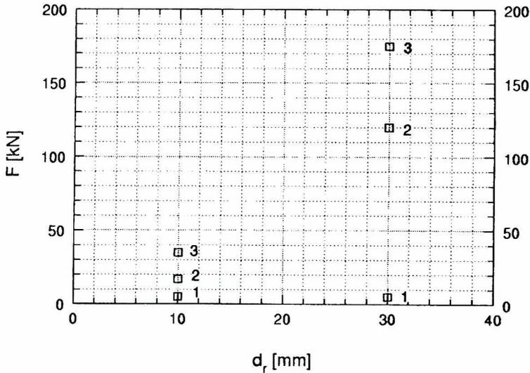
Figure 2. Pull-out force  $F$  versus the diameter of the steel anchor rod  $d_r$  (1. smooth anchor rod, 2. screw-threaded anchor rod, 3. very rough anchor rod)
