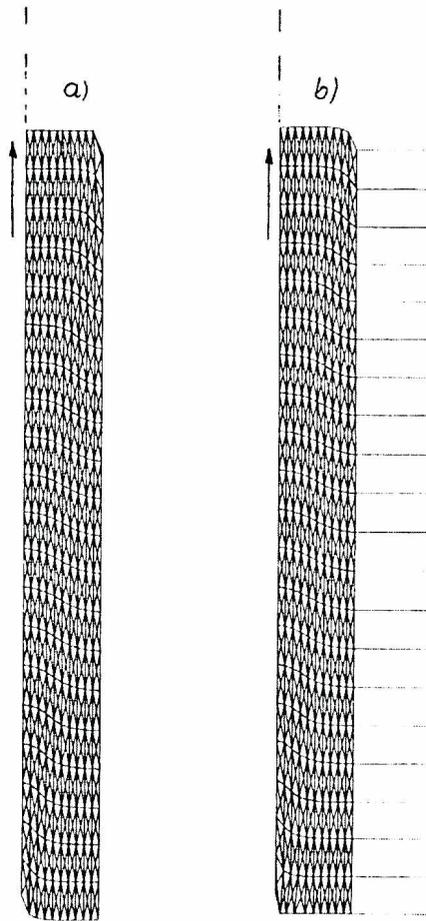
**Figure 8.** Deformed FE-meshes (plane strain,  $d_{50} = 0.5$  mm,  $e_0 = 0.60$ ): a)  $k = \infty$ , b)  $k = 10000$  kN/m
