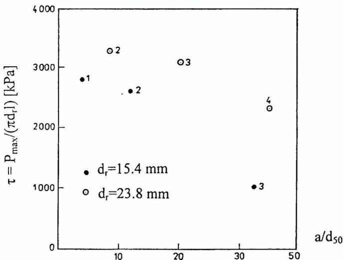
Figure 3. Mean shear stress  $\tau$  along the shaft versus the ratio  $a/d_{50}$  (1. fine gravel, 2. coarse sand, 3. medium sand, 4. fine sand).  $P$  – pull-out force,  $d_r$  – rod diameter,  $l$  – rod length,  $a$  – width of the space between the rod and the borehole wall,  $d_{50}$  – mean grain diameter
