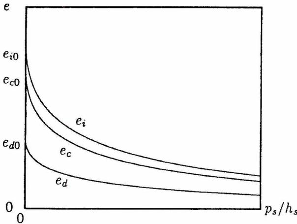
Figure 4. Pressure dependence of void ratios
