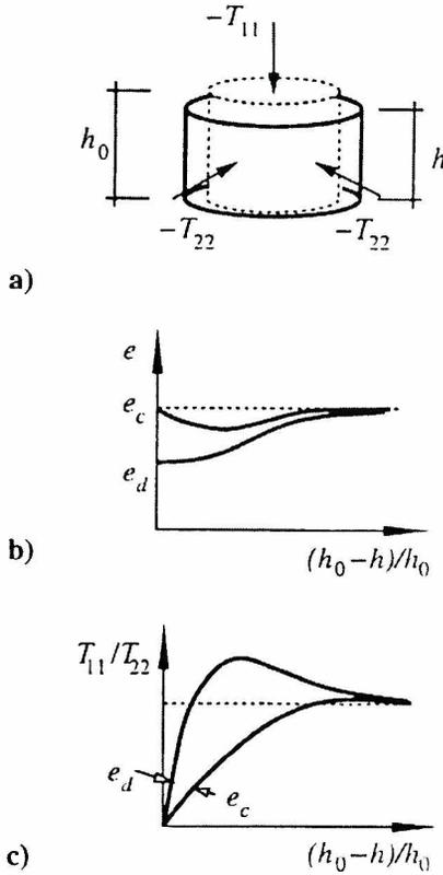
Figure 2. Cylindrical compression with constant mean pressure
