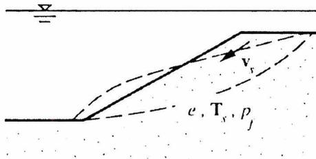
Figure 9. Slope collapse with undrained saturated material
