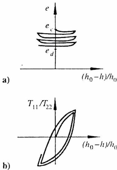
Figure 3. Effect of cyclic changes of height of a cylinder under constant mean pressure
