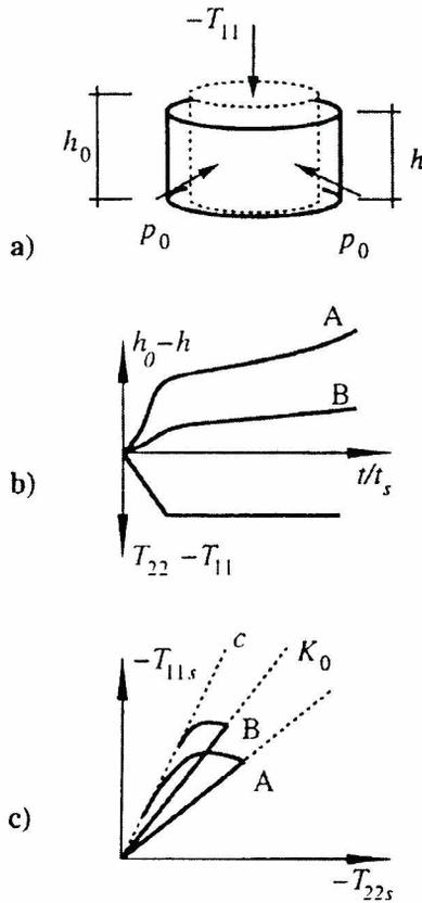
Figure 7. Creep without drainage
