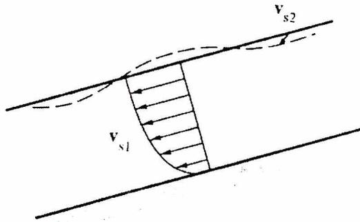
Figure 10. Instability of a creeping slope
