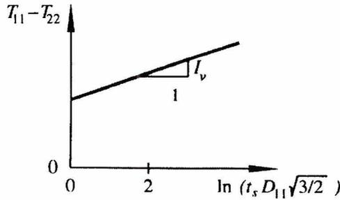
Figure 5. Drained cylindrical compression at critical states with different stretching rates
