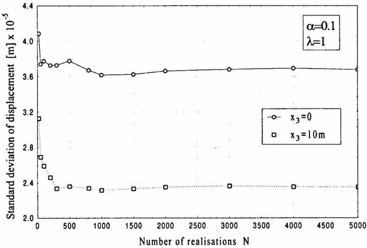
Figure 8. Standard deviation of vertical displacement vs. number of realisations
