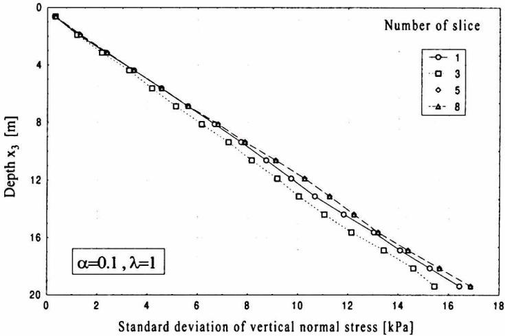
Figure 4. Change of standard deviation of vertical normal stress with depth, for different slices
