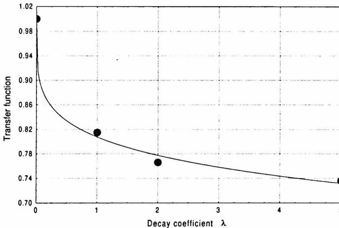
**Figure 13.** Transfer function between standard deviations of vertical displacement in the 2-D and 3-D states
