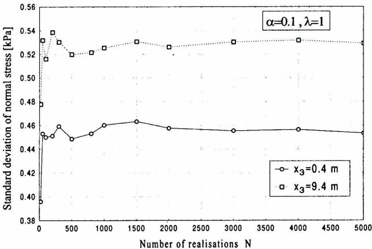
Figure 9. Standard deviation of vertical normal stress vs. number of realisations
