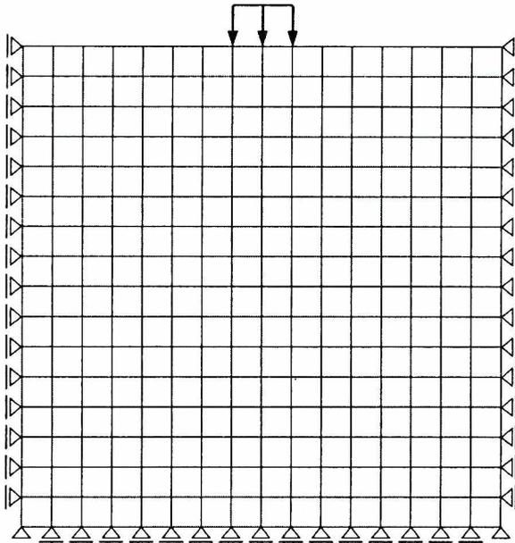
*Figure 1. Finite element mesh applied in 2-D analysis*
