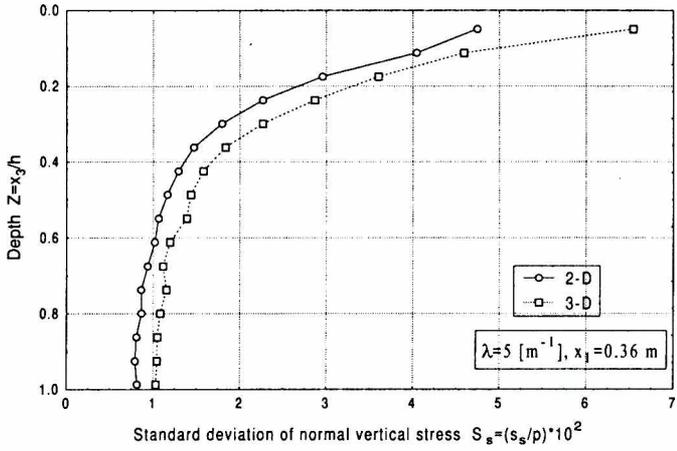
Figure 11. Standard deviation of normal vertical stress vs. depth
