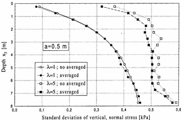
Figure 5. Change of standard deviation of vertical normal stress with depth for mesh spacing  $a=0.5$  m
