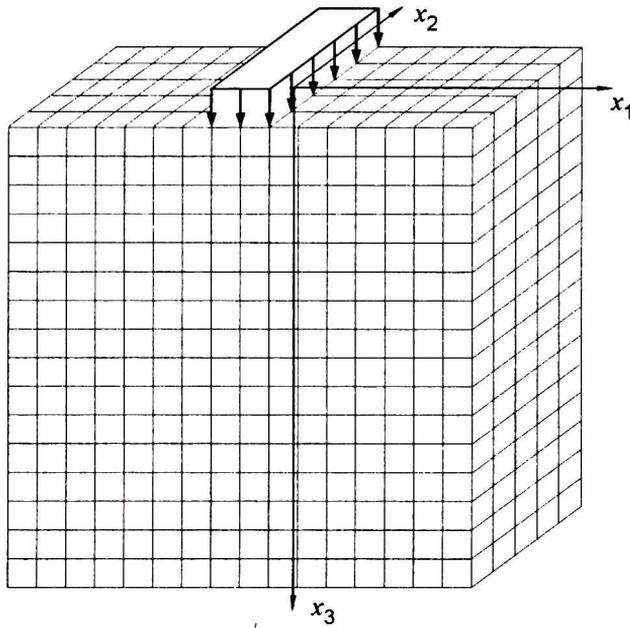
Figure 2. Finite element mesh applied in 3-D analysis
