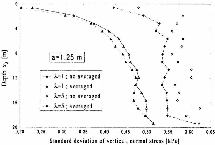
Figure 6. Change of standard deviation of vertical normal stress with depth for mesh spacing  $a=1.25$  m
