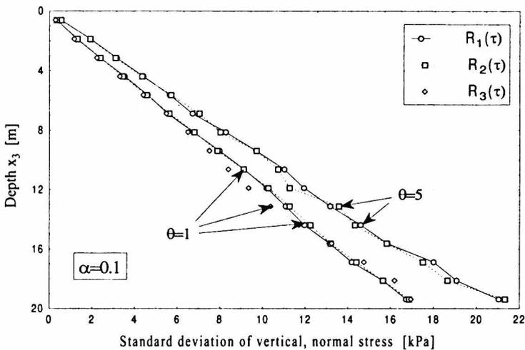
Figure 7. Change of standard deviation of vertical normal stress with depth for different correlation functions
