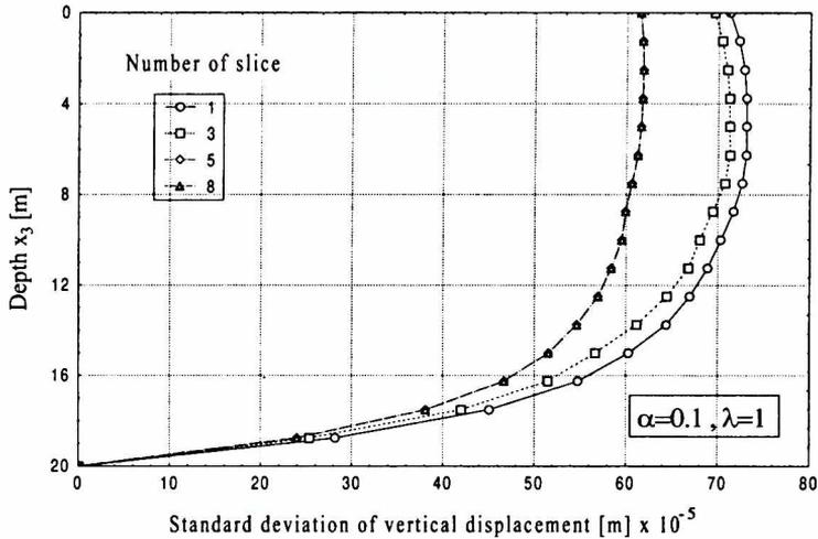
Figure 3. Change of standard deviation of vertical displacement with depth, for different slices
