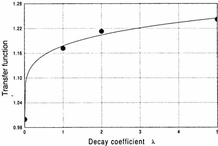
Figure 14. Transfer function between standard deviations of normal vertical stress in the 2D and the 3D states
