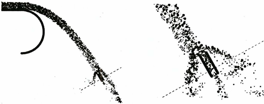
Figure 19. a) Iron ore sampling from a conveyor belt, b) ore passing through the sample cutter
