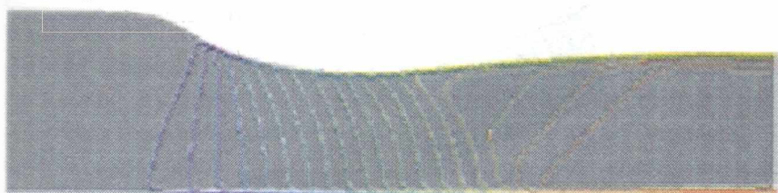
Figure 15. An example of 2-D simulation of nozzle flow with a shock wave
