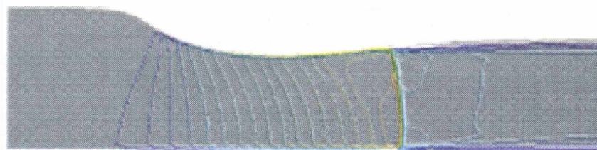
Figure 16. 2-D nozzle flow for different outlet pressure: a) low outlet pressure - full expansion, b) increased outlet pressure, shock upstream Mach number M = 1.47 , c) further increased outlet pressure, shock upstream Mach number M = 1.35
