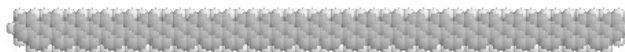
Figure 11. A model C-300 molecule (carbon-graphite strip): large balls stand for carbon atoms, while small ones – for hydrogen atoms
