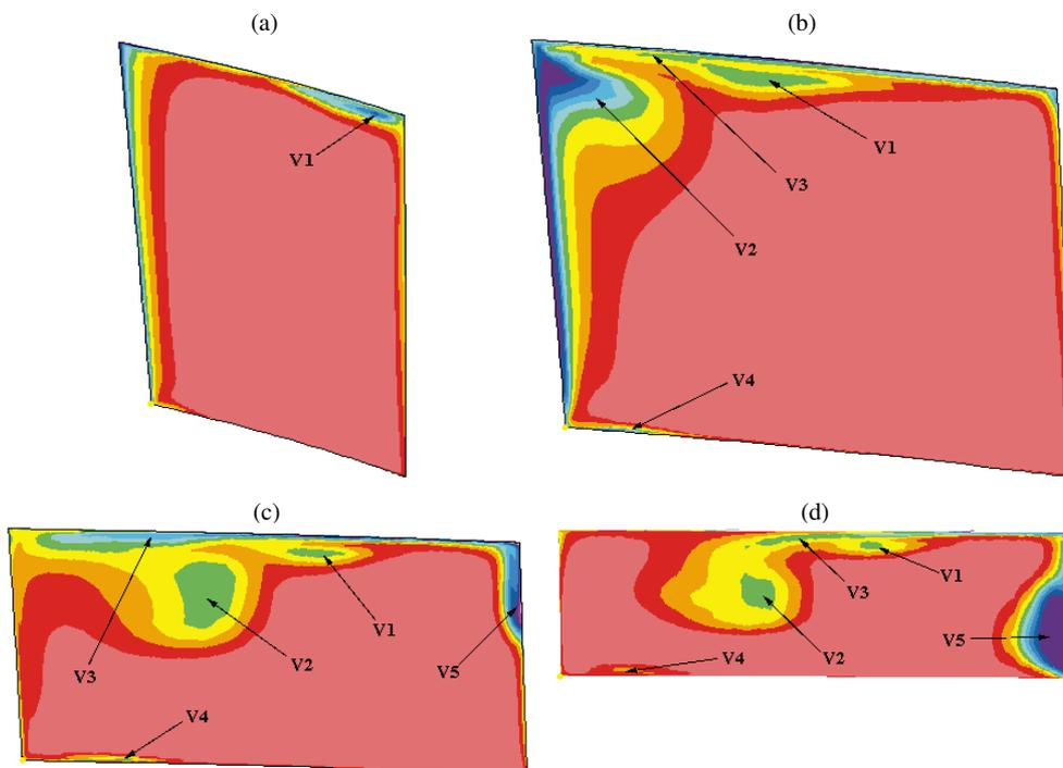
**Figure 10.** Entropy function contours for cross-flow sections of rotor (percentage of chord):
