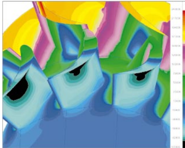
Figure 28. Calculated pressure distribution for a certain runner position
