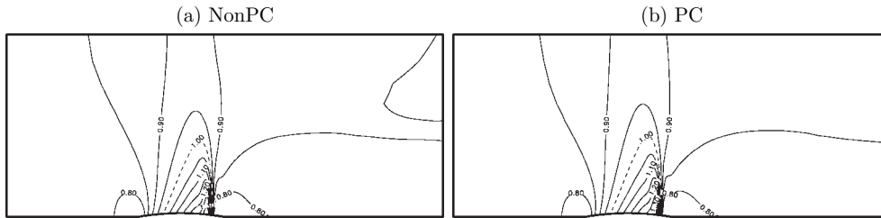
Figure 2. Calculated Mach number contours of the transonic Ni-Bump test case ( Ma_{is} = 0.85 ) using the non-preconditioned (NonPC) and the preconditioned (PC) scheme
