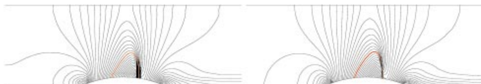
Figure 5. GAMM channel: Iso-Mach lines; TVD MC (left), Osher implicit method on adapted grid (right)
