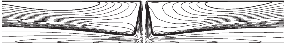
Figure 13. Isolines of velocity for 2D jet, linear (left) and non-linear (right) SST model
