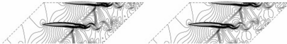
Figure 7. WENO scheme, 50 000 time steps (left), 50 200 time steps (right)
