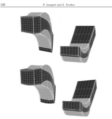
Figure 3. HPTS – a view on the computational grid (coarse grid) of stator (left) and rotor (right) of the original (top) and final (bottom) stage
