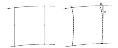
Figure 4. HPTS – original (left) and final (right) shape of stator blades in circumferrential view – positive  $\Delta x$  refers to the direction of rotation (clockwise)
