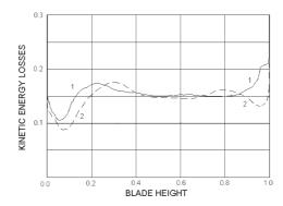
Figure 2. GTS – span-wise distribution of stage losses including the exit energy before (1) and after (2) optimisation
