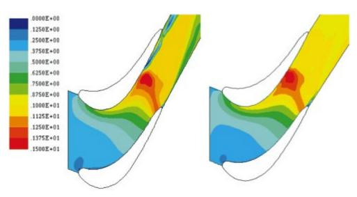
Figure 1. GTS – Mach number contours in the rotor 10% of the blade span from the tip before (left) and after (right) optimisation
