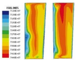
Figure 6. HPTS – total pressure contours behind the rotor before (left) and after (right) optimisation
