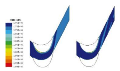
Figure 7. HPTS – entropy function contours in the rotor 8% blade span from the root before (left) and after (right) optimisation
