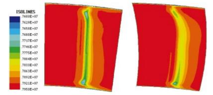
Figure 5. HPTS – total pressure contours downstream of the stator before (left) and after (right) optimisation
