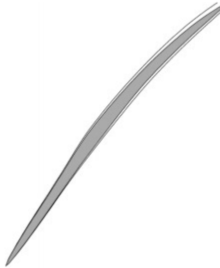
Figure 21. Subtraction of the boundary layer: mean section
