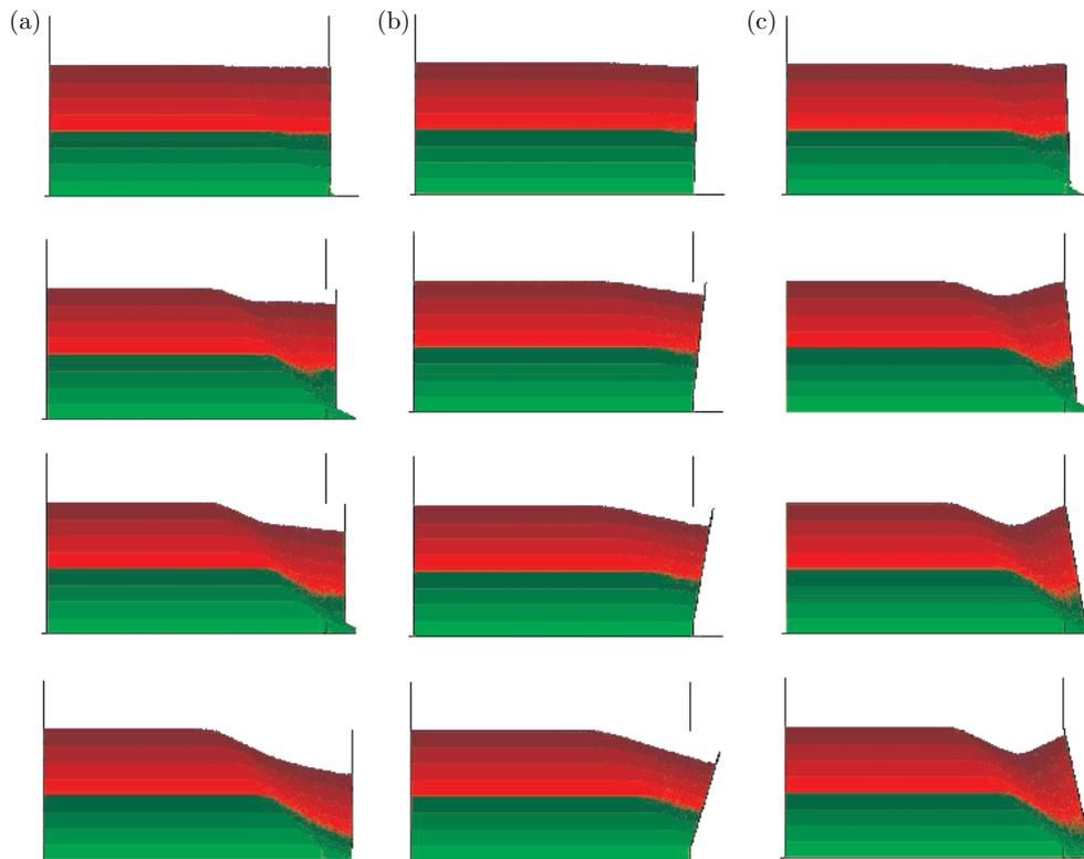
**Figure 4.** Flow patterns during an active mode of a retaining wall: (a) translating wall, (b) wall rotating around the top, (c) wall rotating around the bottom (migration scheme of Figure 1a,  $p_1 = 0.45$ ,  $p_2 = 0.23$ ,  $p_3 = 0.05$ ,  $p_4 = p_5 = 0.14$ )
