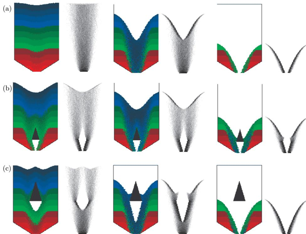
**Figure 5.** Flow patterns and distribution of flow rate during granular flow: (a) in a silo without insert, (b) and (c) in a silo with insert (migration rule of Figure 1a,  $p_1 = p_5 = 0.30$ ,  $p_2 = p_4 = 0.15$ ,  $p_3 = 0.05$ )
