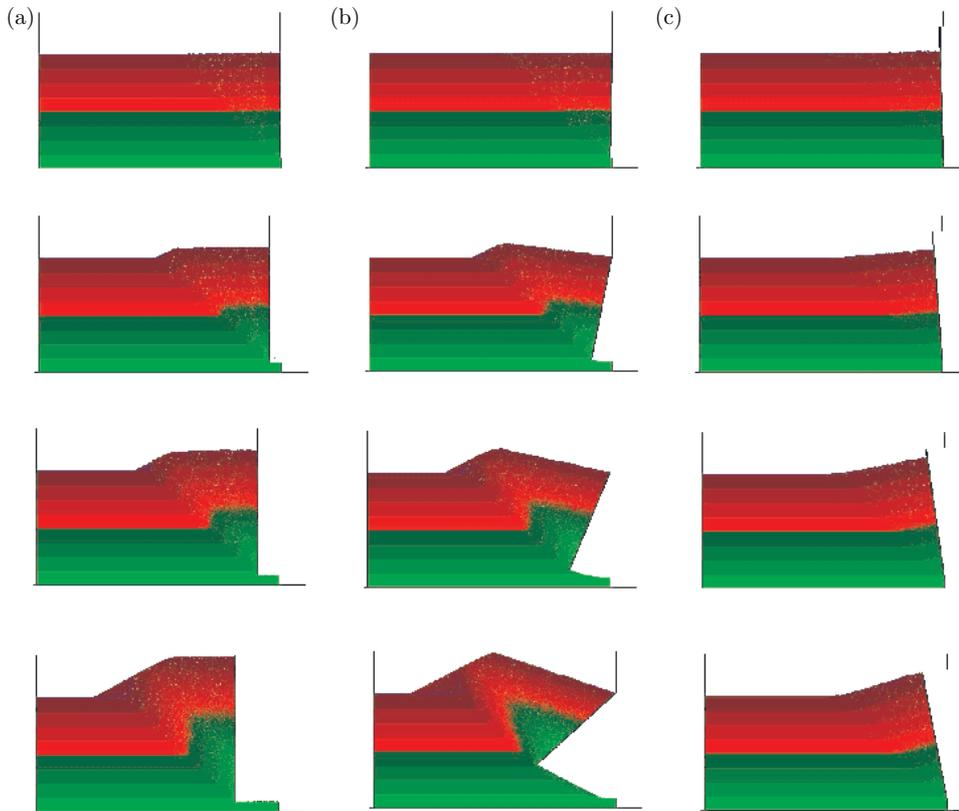
**Figure 3.** Flow patterns during a passive mode of a retaining wall: (a) translating wall, (b) wall rotating around the top, (c) wall rotating around the bottom (migration scheme of Figure 1b,  $p_1 = p_2 = 0.33$ ,  $p_8 = 0.33$ ,  $p_3 = p_4 = p_5 = p_6 = p_7 = 0$ )
