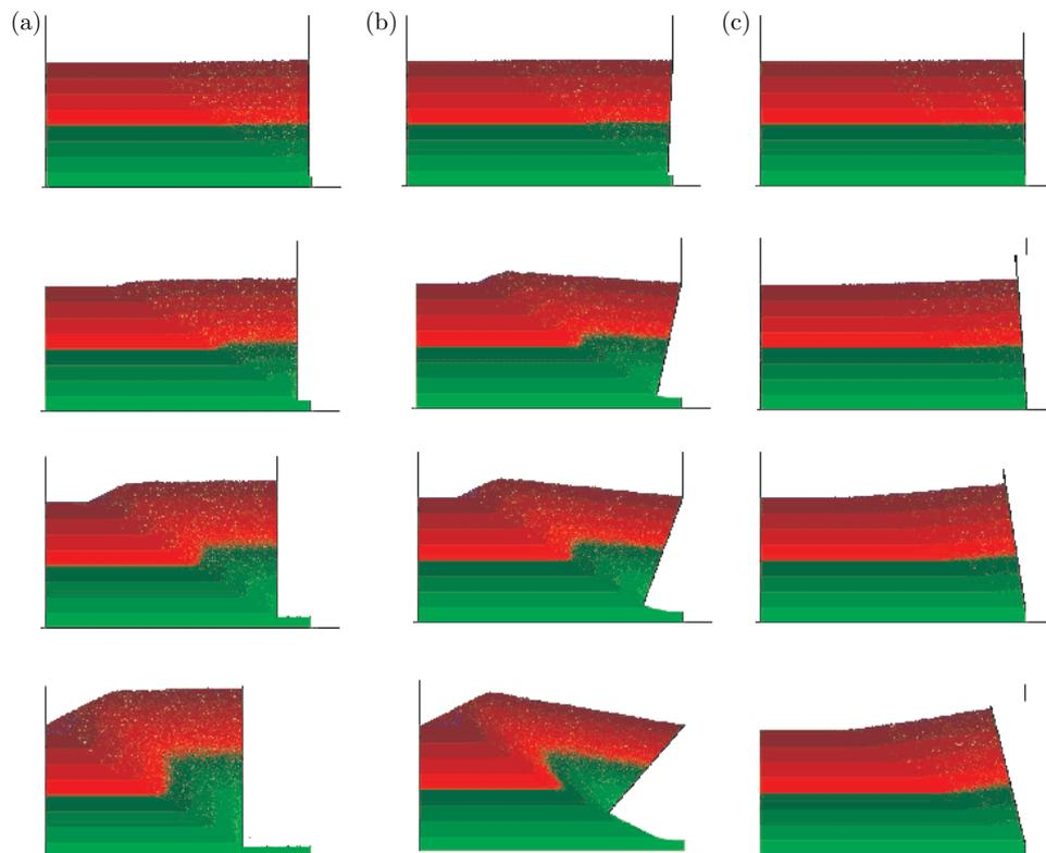
**Figure 2.** Flow patterns during a passive mode of a retaining wall: (a) translating wall, (b) wall rotating around the top, (c) wall rotating around the bottom (migration scheme of Figure 1b,  $p_1 = p_2 = 0.25$ ,  $p_8 = 0.50$ ,  $p_3 = p_4 = p_5 = p_6 = p_7 = 0$ )
