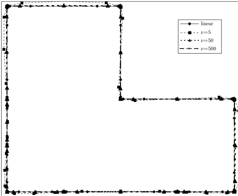
Figure 2. Living room defined by linear segments and  $\nu$ -spline curves for different curvature coefficients
