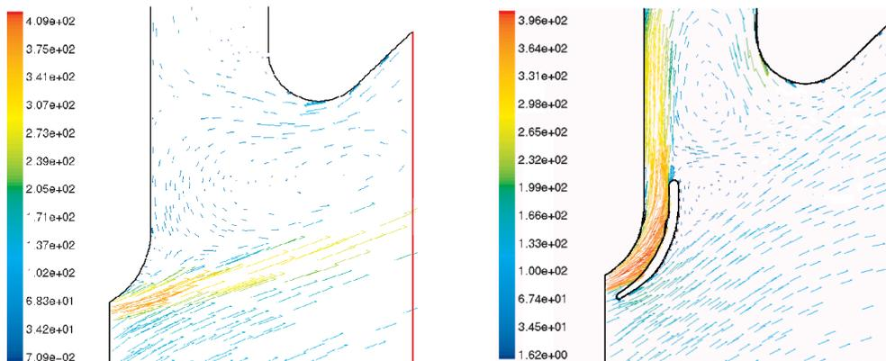
Figure 10. Velocity vectors before and after modernisation
