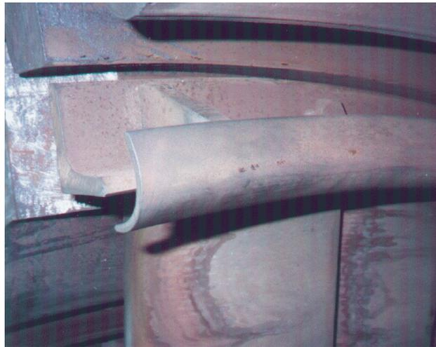
Figure 4. Ring inside the turbine flow path after six years of operation
