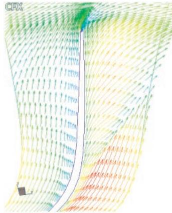
**Figure 12.** Velocity vectors view on the S1 surface (blade profile mark in the center of the drawing) close to the blade tip. At the suction side, secondary flow vortex clearly visible ( $m = 16 \text{ kg/s}$ )
