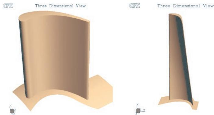
**Figure 25.** Two different kinds of rotor blades: left – cylindrical, right – twisted
