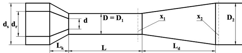
Figure 1. A diagram of an air-air ejector according to [1]
