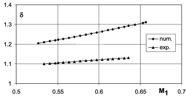
Figure 6. Variation of the pressure rise coefficient in the diffuser as a function of inlet velocity
