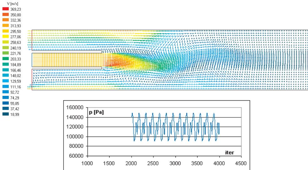
Figure 9. An example of flow with Hopf bifurcations (top); pressure–iterations diagram (bottom)
