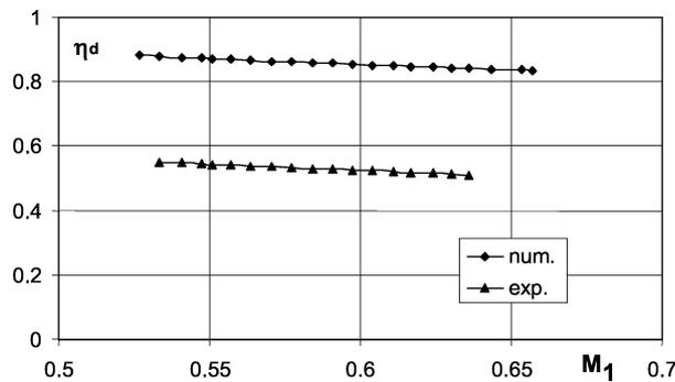
Figure 7. Diffuser efficiency as a function of inlet velocity
