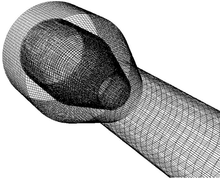
**Figure 3.** A fragment of the calculation grid of the modelled ejector, a 3D case
