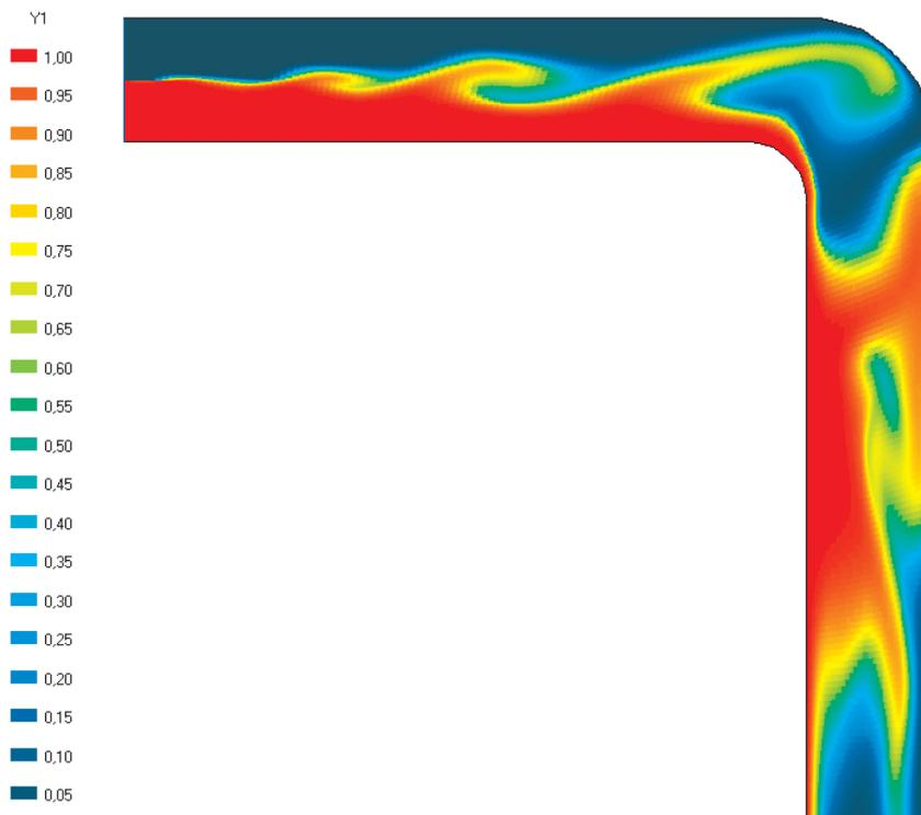
Figure 12. An example of whirls in the boundary zone during parallel flow of two components [4]
