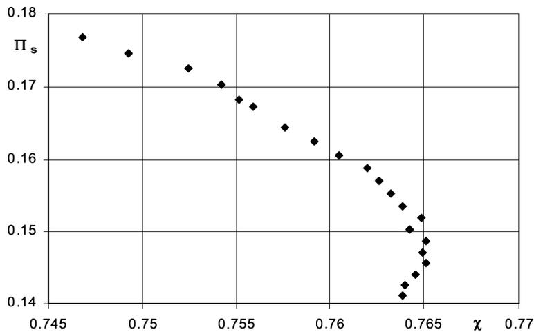
Figure 8. Ejector performance characteristics  $\Pi_s = f(\chi)$  obtained by numerical simulation
