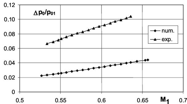
Figure 5. The relative total pressure drop in the diffuser as a function of inlet velocity
