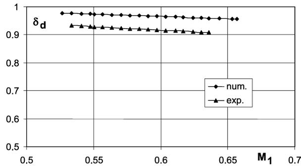
Figure 4. Variation of the pressure loss coefficient as a function of inlet velocity
