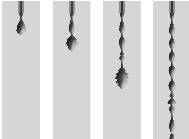
Figure 5. Subsequent stages of simulation of unstable core-annular flow; \bar{w}_A/\bar{w}_B = 21.6 , Re = 0.106 , \mu_A/\mu_B = 0.00231 , \rho_A/\rho_B = 1.023
