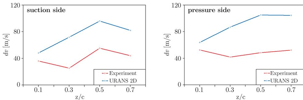
Figure 5. Velocity fluctuation amplitudes in the model turbine rotor passage
