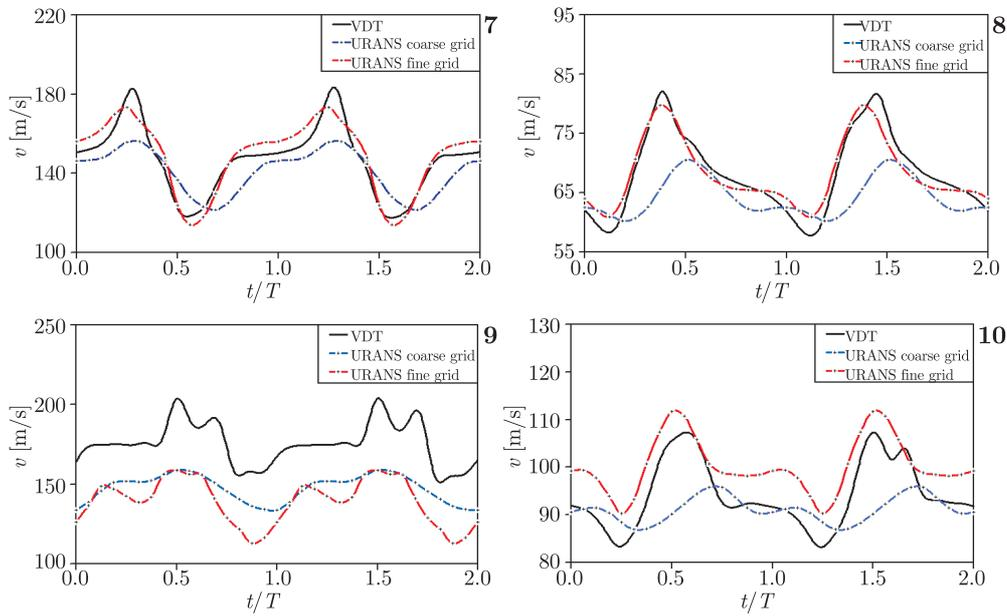
**Figure 6 – continued.** Time-histories of velocity fluctuations in the real turbine rotor passage
