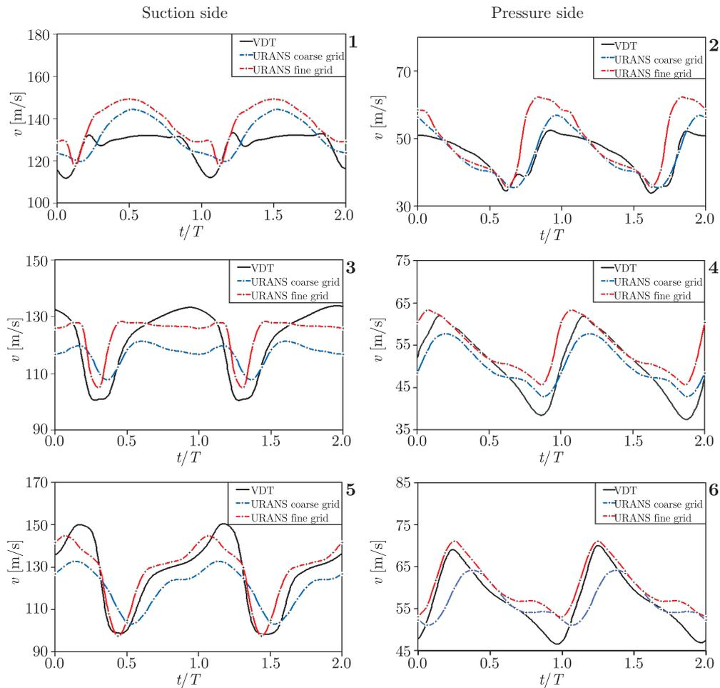
**Figure 6.** Time-histories of velocity fluctuations in the real turbine rotor passage
