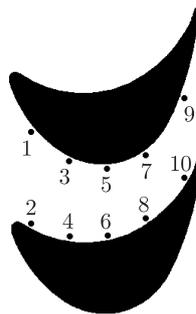
**Figure 2.** Velocity recording points in the rotor passage
