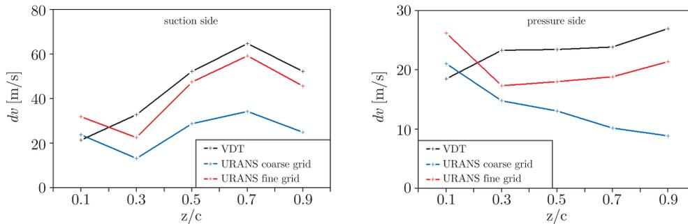
Figure 8. Velocity fluctuation amplitudes in the real turbine rotor passage
