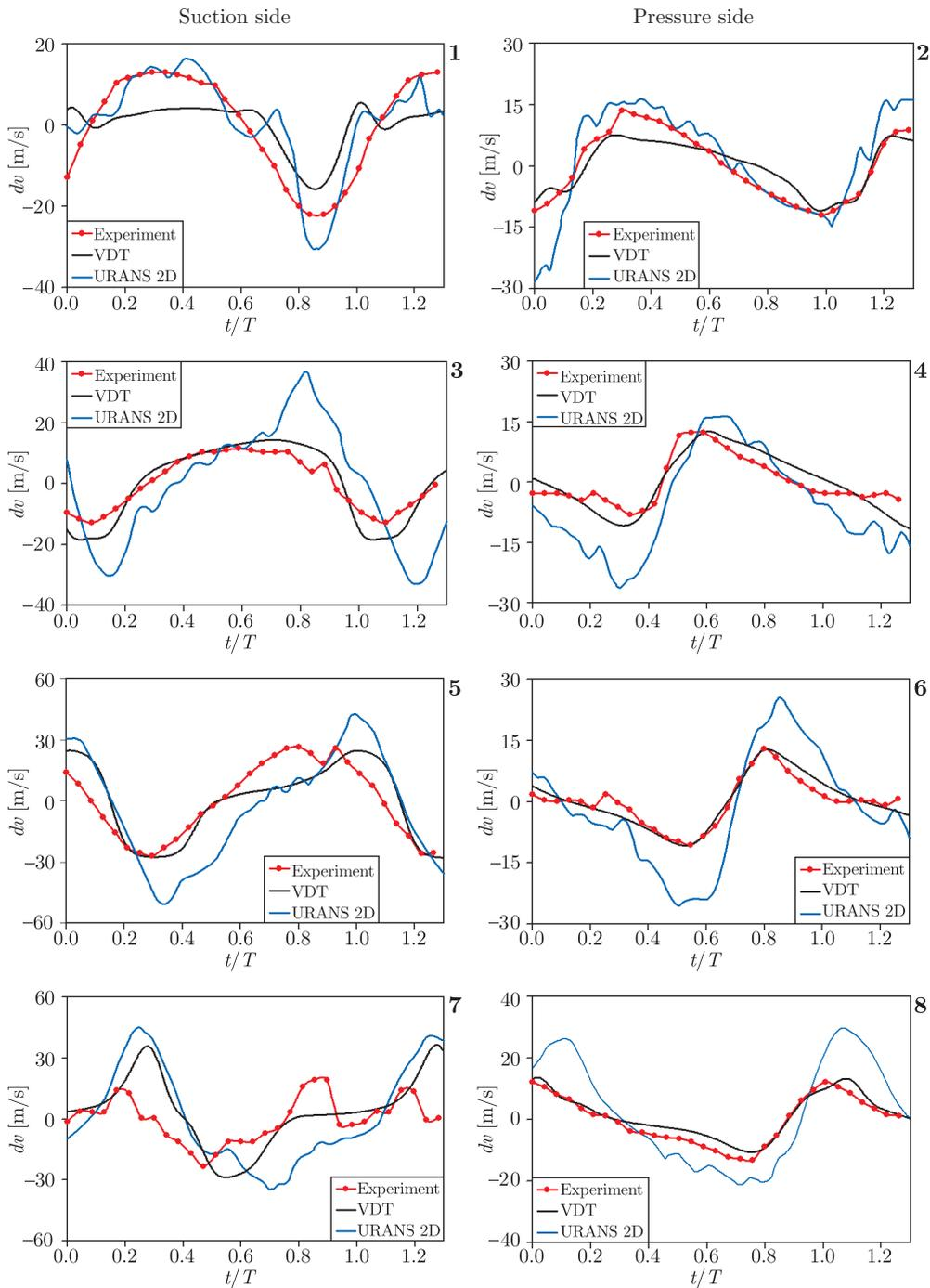
**Figure 3.** Time-histories of velocity fluctuations in the model turbine rotor passage
