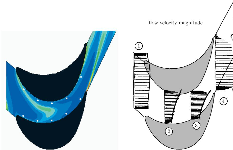
**Figure 7.** Locations of measuring points against instantaneous wake flow pattern (left) and flow velocity profiles in the rotor passage (right)
