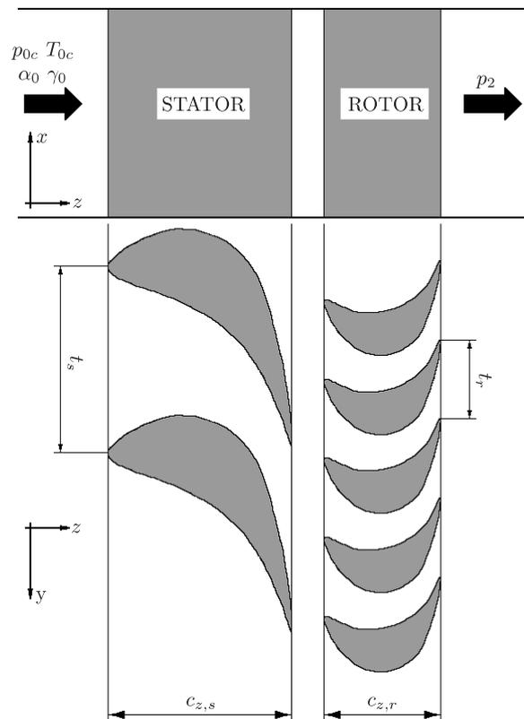
**Figure 1.** Turbine stage geometry and flow parameters assumed in URANS calculations
