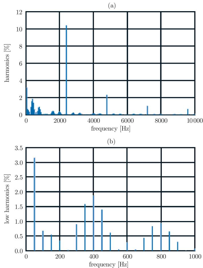
**Figure 6.** Harmonics (a) and low harmonics (b) of the unsteady axial force (regime 4, top cross-section,  $m_{\text{extr}} = 15.38 \text{ kg/s}$ ,  $A_0 = 42.0481 \text{ N}$ )
