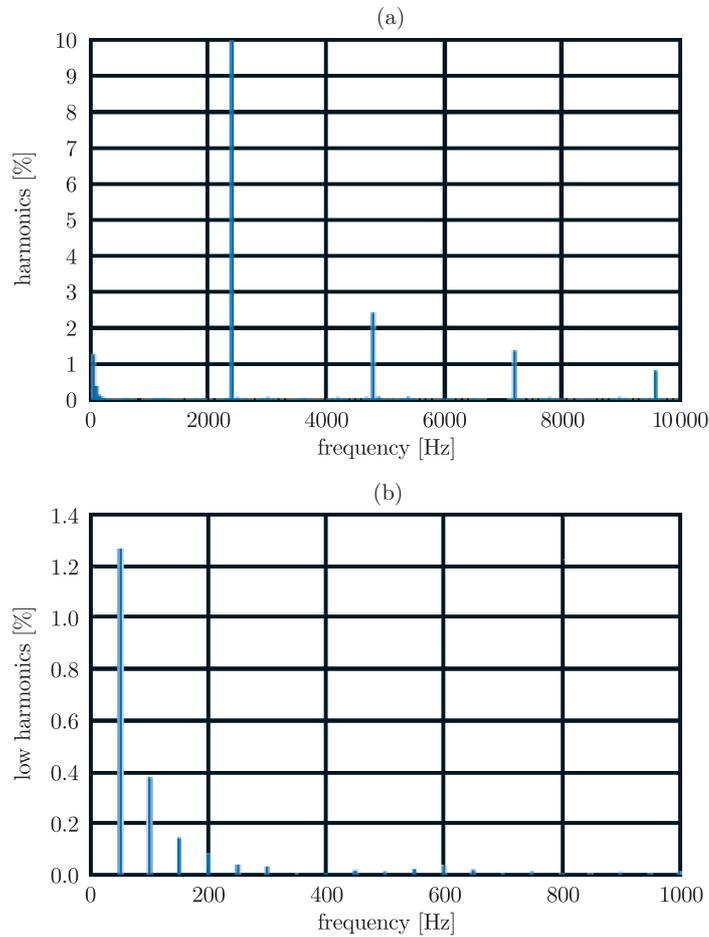
**Figure 5.** Harmonics (a) and low harmonics (b) of the unsteady axial force (regime 1, top cross-section,  $m_{\text{extr}} = 5.42 \text{ kg/s}$ ,  $A_0 = 32.044 \text{ N}$ )
