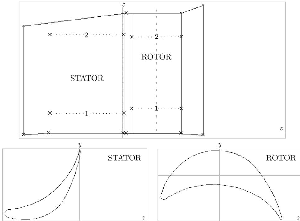
**Figure 4.** Cross-sections of the stage (top) and the stator and rotor blades (bottom)
