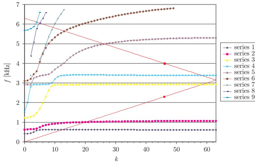
Figure 7. Interference diagram of the bladed disc
