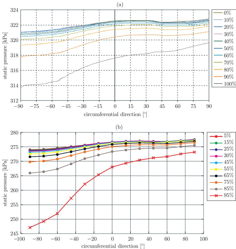
**Figure 3.** Pressure distribution behind the rotor blades: (a) for regime 1 ( $m_{\text{extr}} = 5.42 \text{ kg/s}$ ); (b) for regime 4 ( $m_{\text{extr}} = 15.38 \text{ kg/s}$ )
