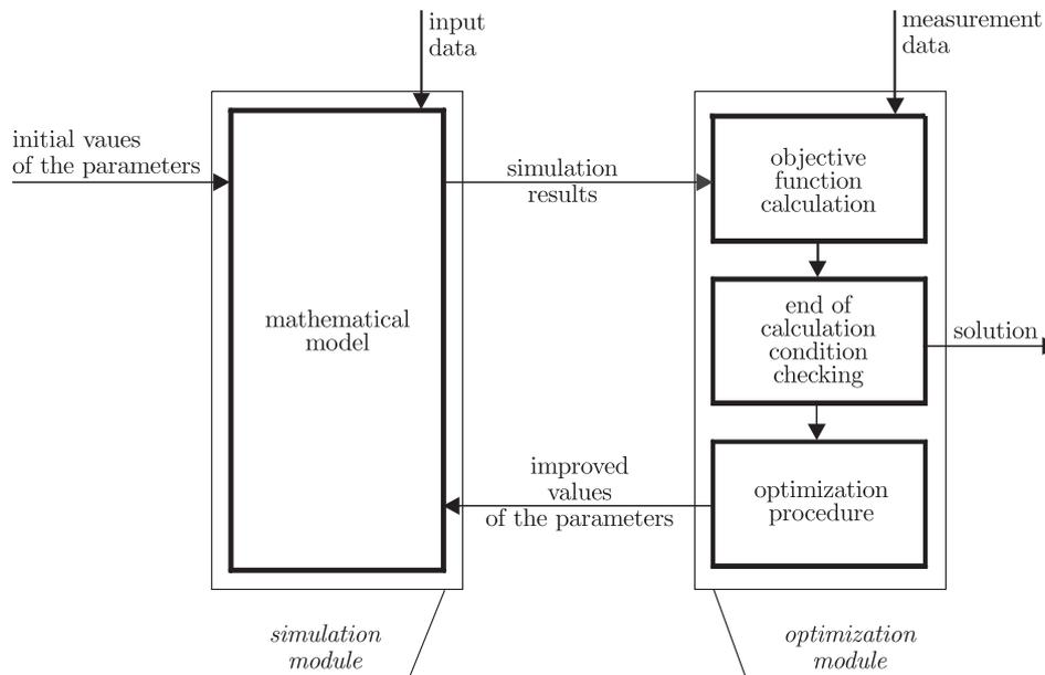
**Figure 1.** Schema of an automatic calibration (optimization) problem
