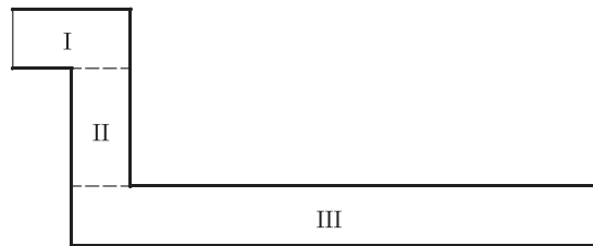
Figure 10. Schematic of a double bent channel domain with three adjacent rectangles
