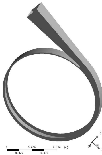
Figure 3. View of spiral outflow collector and outlet diffuser
