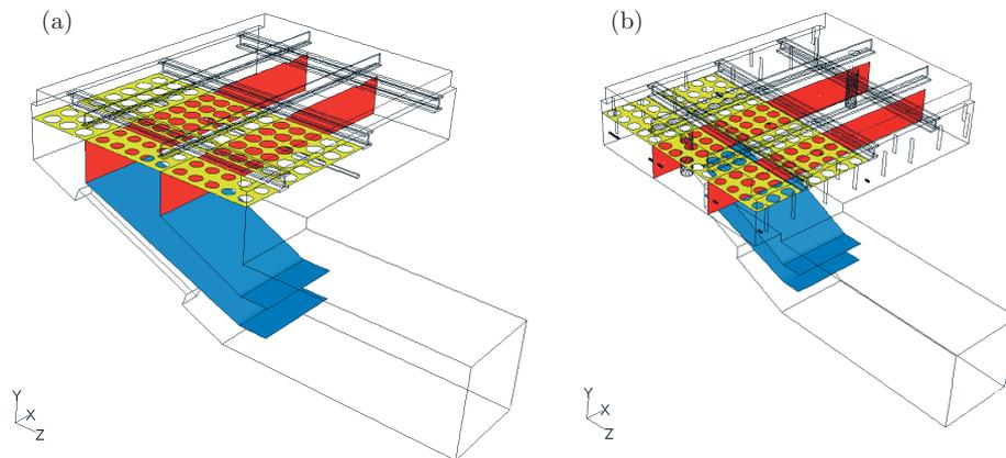
**Figure 6.** The modified geometry of (a) the side windbox and (b) the middle windbox
