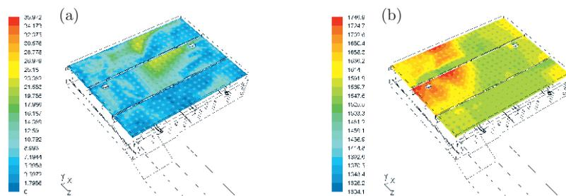
**Figure 5.** (a) The contour-plot velocity field [m/s] and (b) static pressure field [Pa] in the grid space of the middle windbox for 100% MCR
