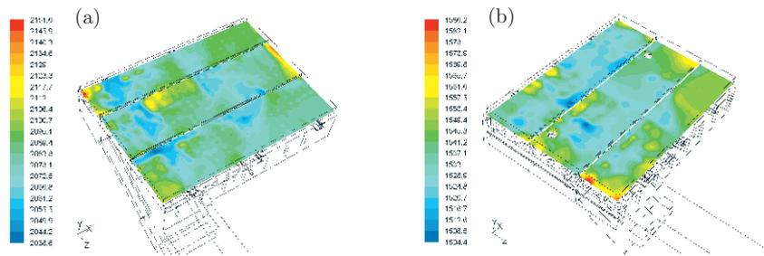
**Figure 9.** Static pressure [Pa] distribution in the grid zone of (a) the side windbox and (b) the middle windbox after upgrading, for 100% MCR
