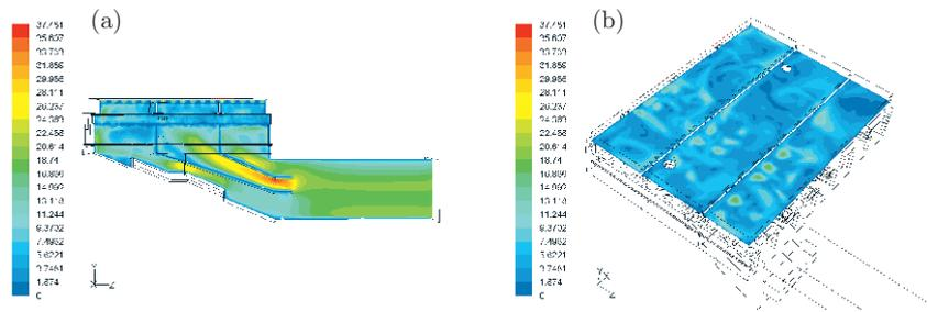
**Figure 8.** Velocity [m/s] distribution in (a) the inlet channel and in (b) the grid zone of the middle windbox after upgrading, for 100% MCR
