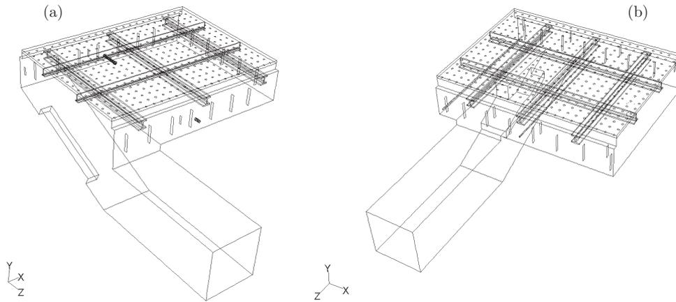
**Figure 3.** Geometry of (a) the side windbox and (b) the middle windbox, as defined in the GAMBIT program
