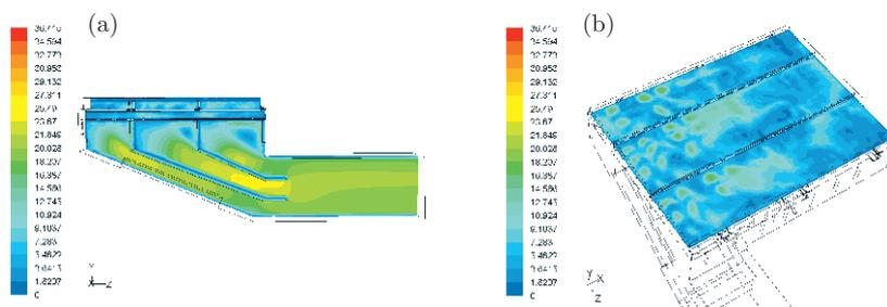
**Figure 7.** Velocity [m/s] distribution in the (a) inlet channel and in (b) the grid zone of the side windbox after upgrading, for 100% MCR
