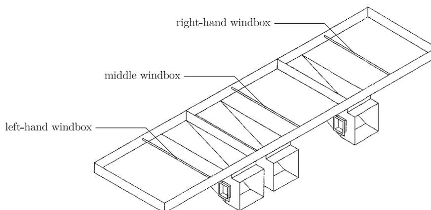
Figure 1. Arrangement of windboxes in the 670 MW<sub>th</sub> power CFB boiler
