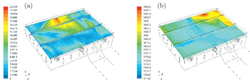
**Figure 4.** (a) The contour-plot velocity field [m/s] and (b) static pressure field [Pa] in the grid space of the side windbox for 100% MCR
