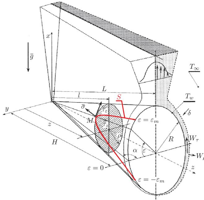
Figure 1. A coordinate system of an isothermal horizontal conical surface transferring heat by free convection [9]
